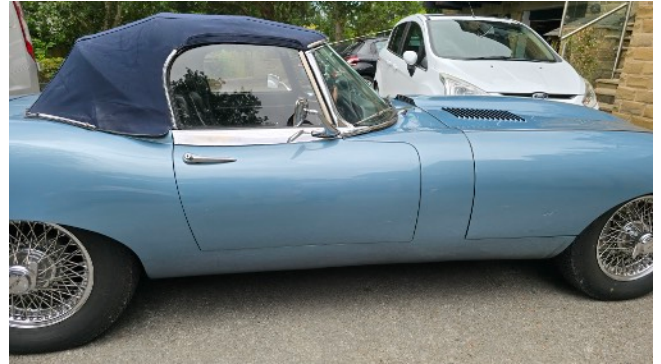
Body and paintwork. Localised previous repair is present forward of the right-hand rear wheel arch.
