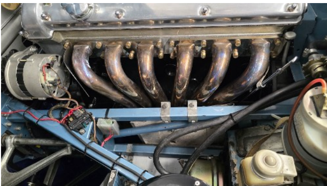
Engine bay showing the tubular exhaust manifolds forming part of the Classic Fabs exhaust installation.
