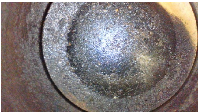
Borescope views of the six combustion chambers and piston crowns. Differences in combustion-deposit patterns are visible between cylinders.
