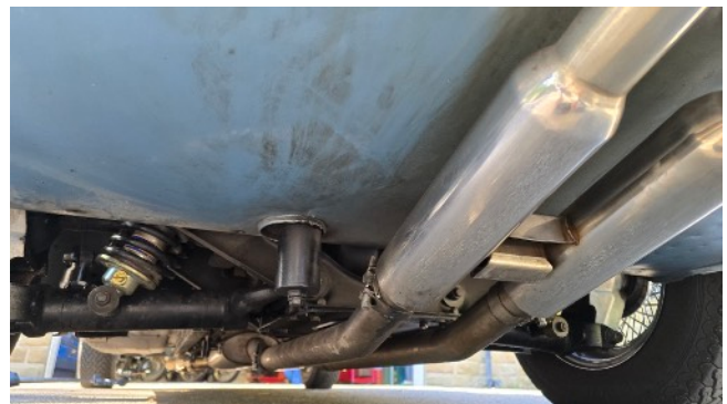
Classic Fabs stainless-steel exhaust system and underside installation.
