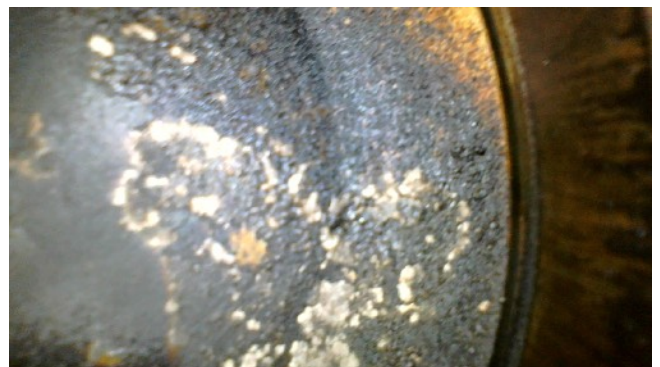
Borescope views of the six combustion chambers and piston crowns. Differences in combustion-deposit patterns are visible between cylinders.
